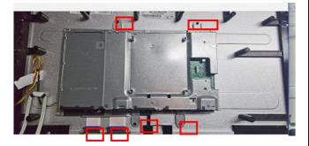
Remove the four screws on the mainframe and then disconnect the FFC cables
