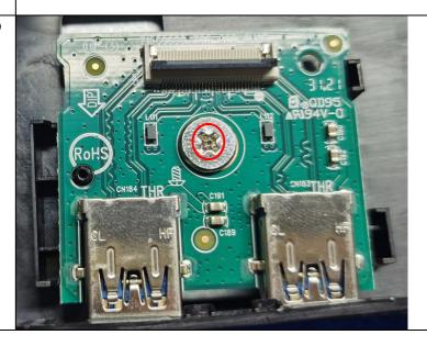
Remove the screw on the usb board
